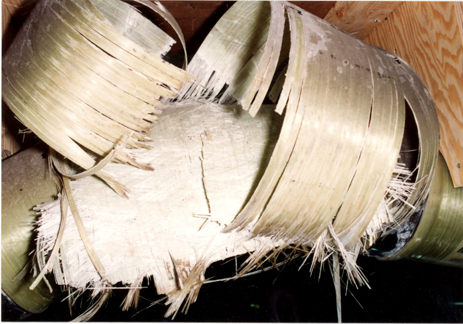
41. View of the top right side of the tank showing the fracture of the composite wrap with the forward end of the tank toward the left side of the photograph
